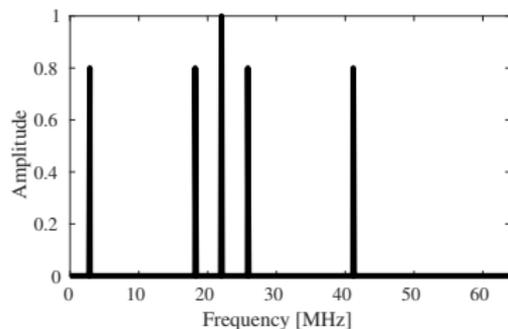
frequency spectrum of APOD DOR tones used in the simulation
