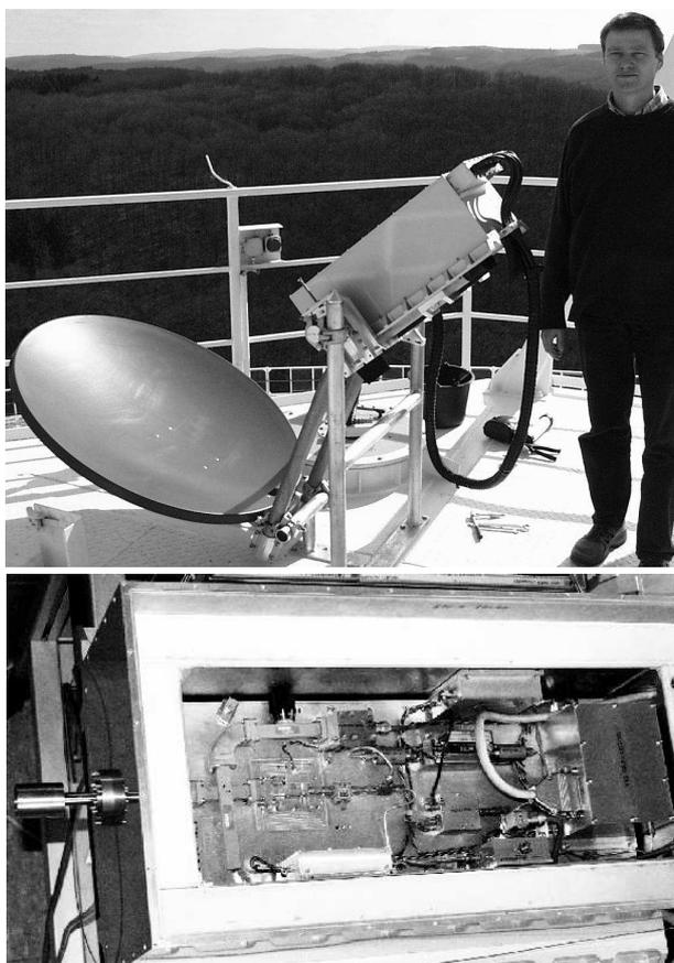
**Fig. 1.** Top: View of the radiometer on top of the primary-focus cabin at Effelsberg. Bottom: Front end opened, showing waveguide components mounted on a temperature-stabilized plate in an insulated box.
