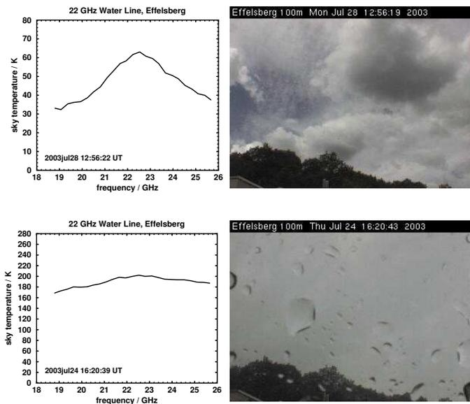
**Fig. 5.** Examples of water line spectra (left) and the corresponding sky conditions (right) measured on 2003 Jul 24 and 28 from the control-building roof in Effelsberg, looking towards azimuth = 330°, elevation = 30°. At the top, one sees fair-weather cumulus and below is during an intense storm with rain.
