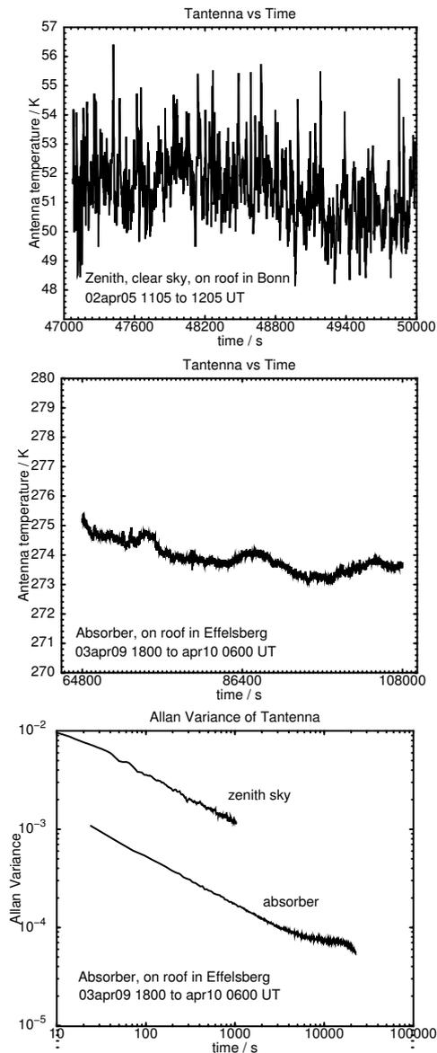
**Fig. 3.** Top left: time series of  $T_{\text{antenna}}$  at zenith on clear blue sky for 1 h shows fluctuations mostly due to atmospheric water vapour. Integration time was 0.3 s per point. Top right: Time series of  $T_{\text{antenna}}$  on an ambient-temperature absorber for 12 h shows much smaller fluctuations, due to gain and absorber temperature changes. Integration time was 0.025 s per point. Bottom: Allan variance of the time series.
