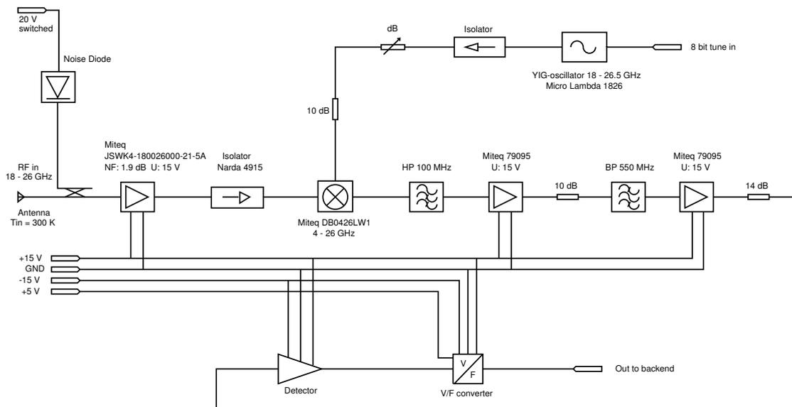
Fig. 2. Block schematic of the front end
