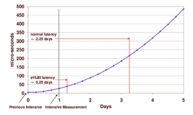
Reducing data latency from 2.25 days to 6 hours results in: Factor of 5 reduction in UT1-UTC prediction uncertainty 40% reduction UT1-UTC prediction errors 7 days out.
