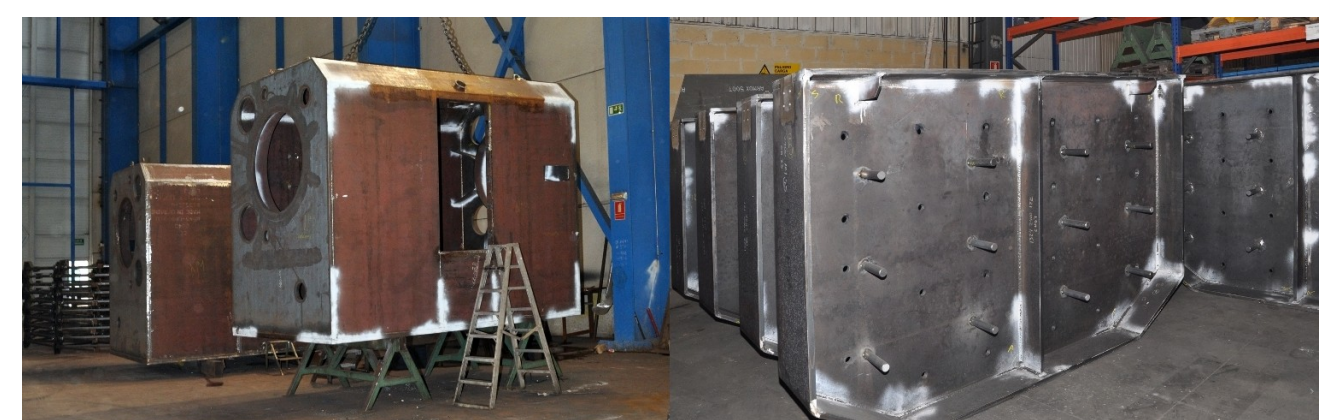
Status of construction of the RAEGE antennas (left: receiver cabins; right: counterweights).
