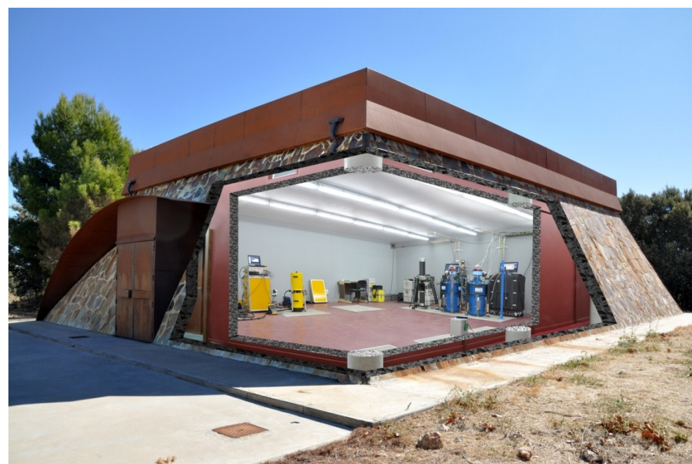
Gravimeter pavilion at Yebes Observatory, with the location of permanent absolute (FG5, A10) and superconducting (GWR/OSG) gravimeters.
