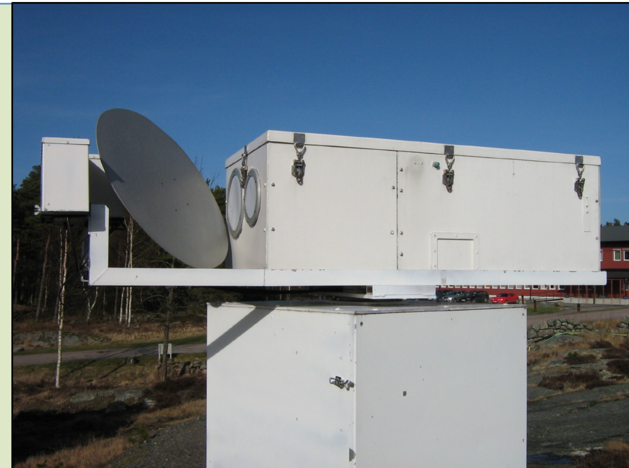
4. The permanently installed microwave radiometer Astrid.
