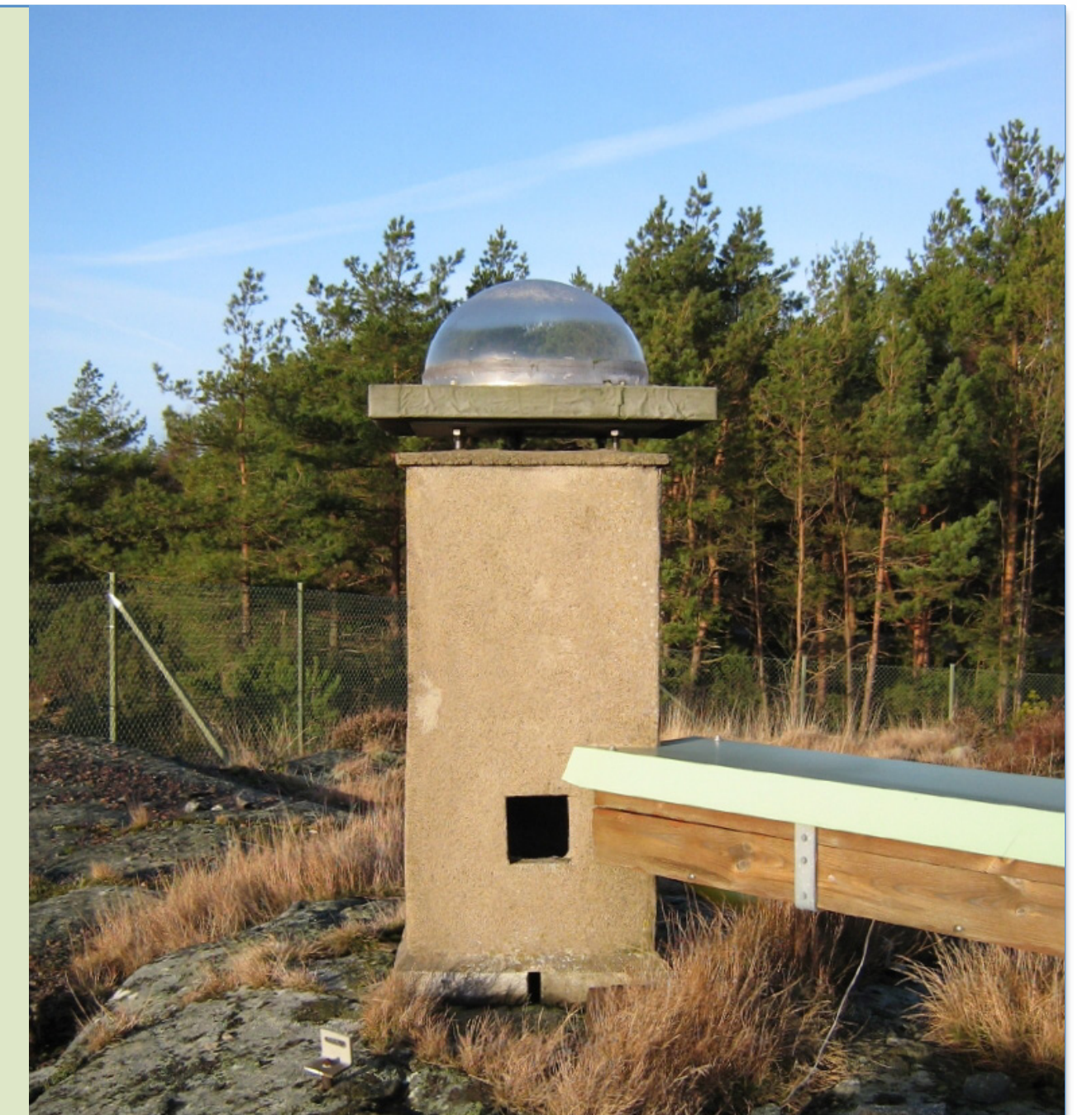
2. The GNSS-monument ONSA built in 1993, part of IGS and SWEPOS.
