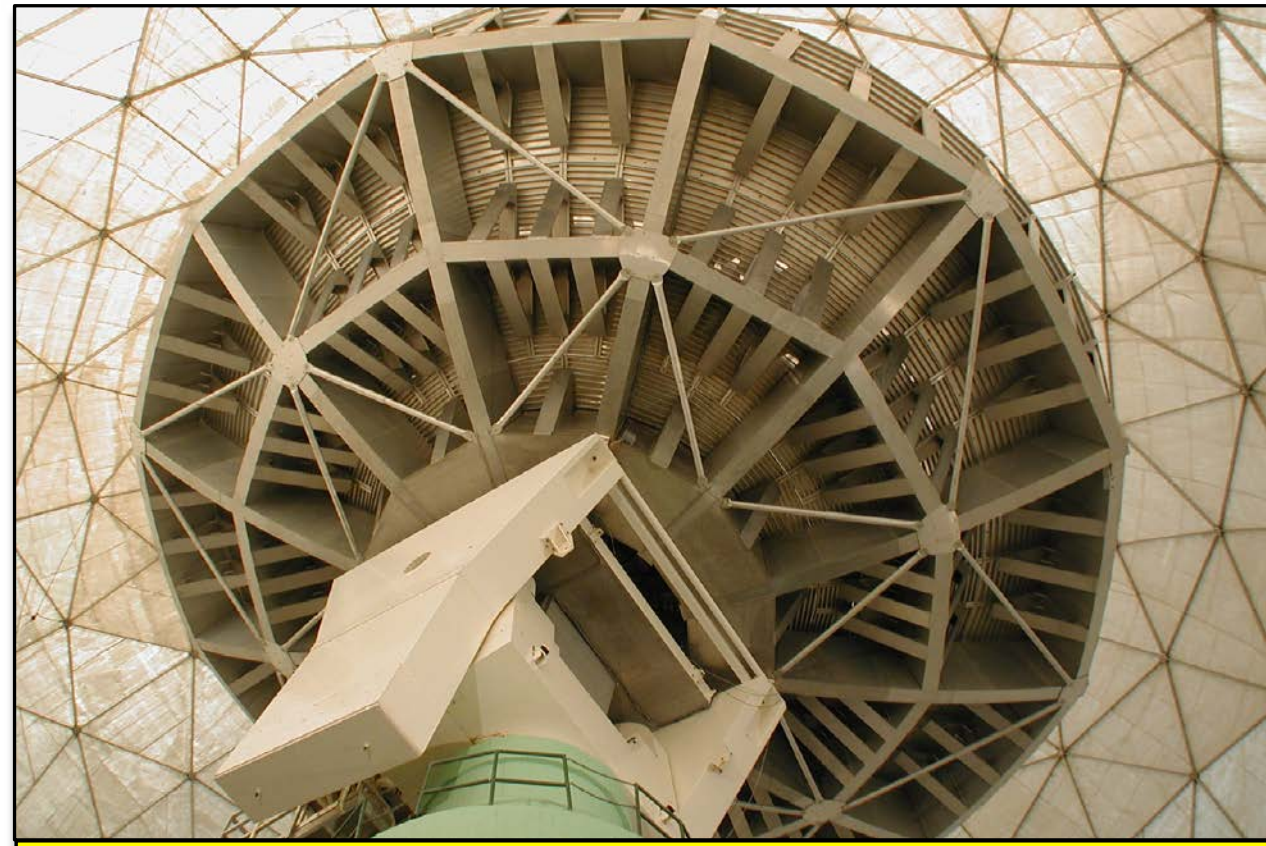
1. The radome enclosed 20 m radio telescope used for geodetic VLBI.
