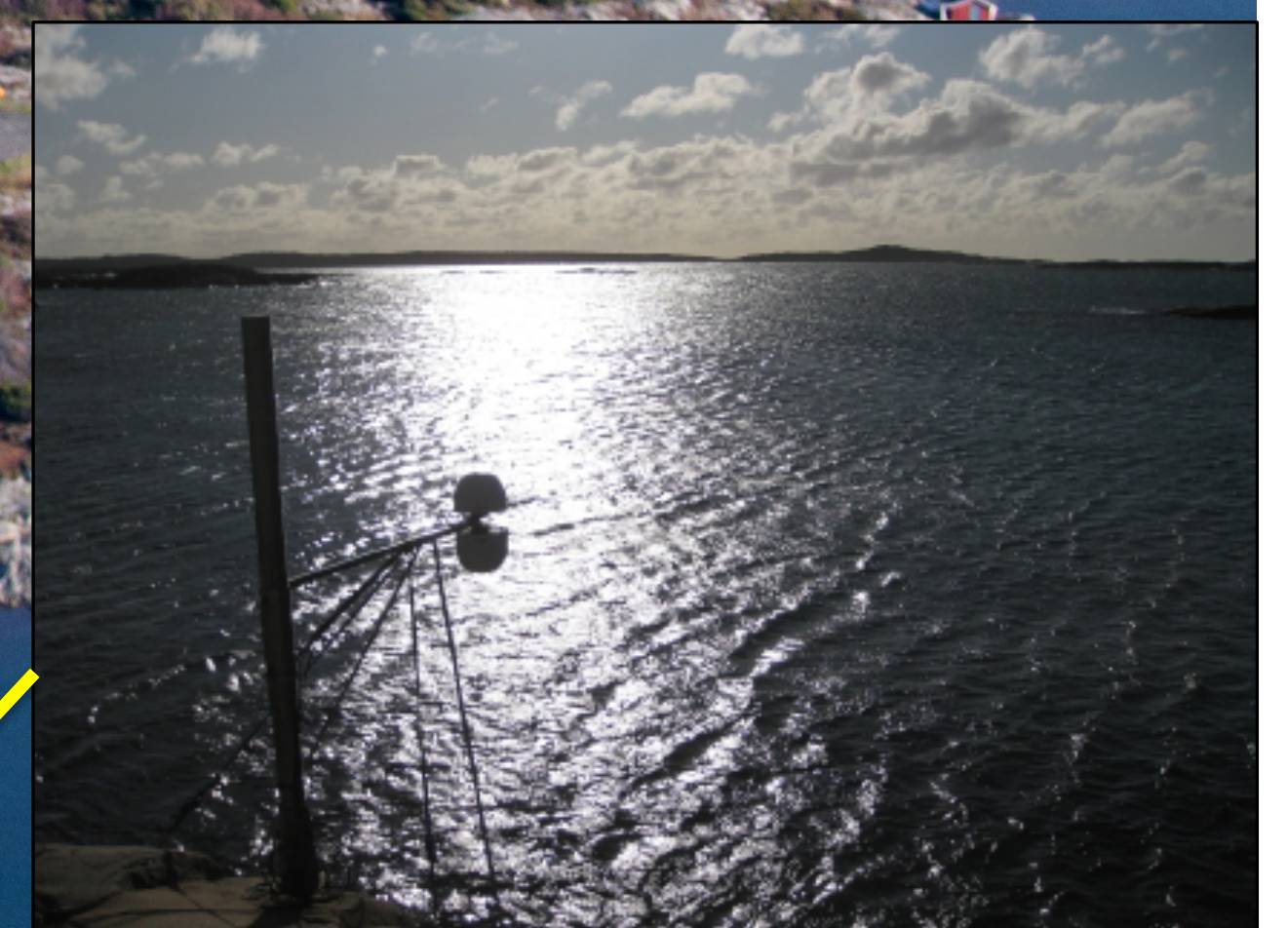
9. The GNSS-based tide gauge operating since 2011.
