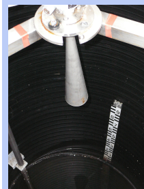
Figure 2. The radar sensor, CS476, operating at 26 GHz.
