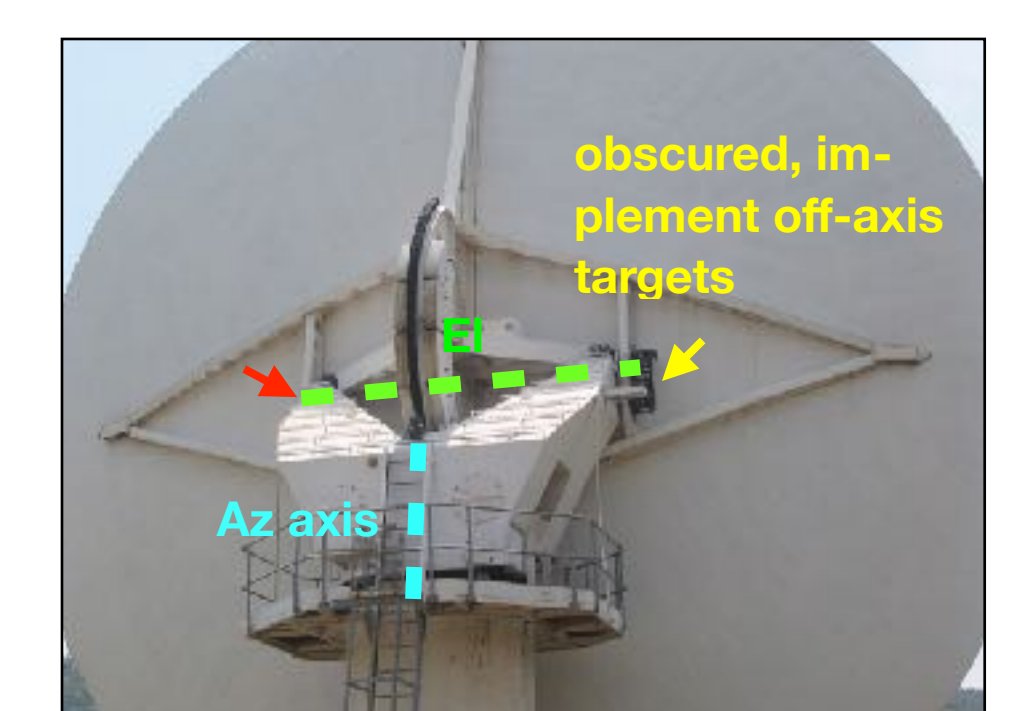
Figure 9: HartRAO 15m az-el mount - rotation axes and prism mounting point.
