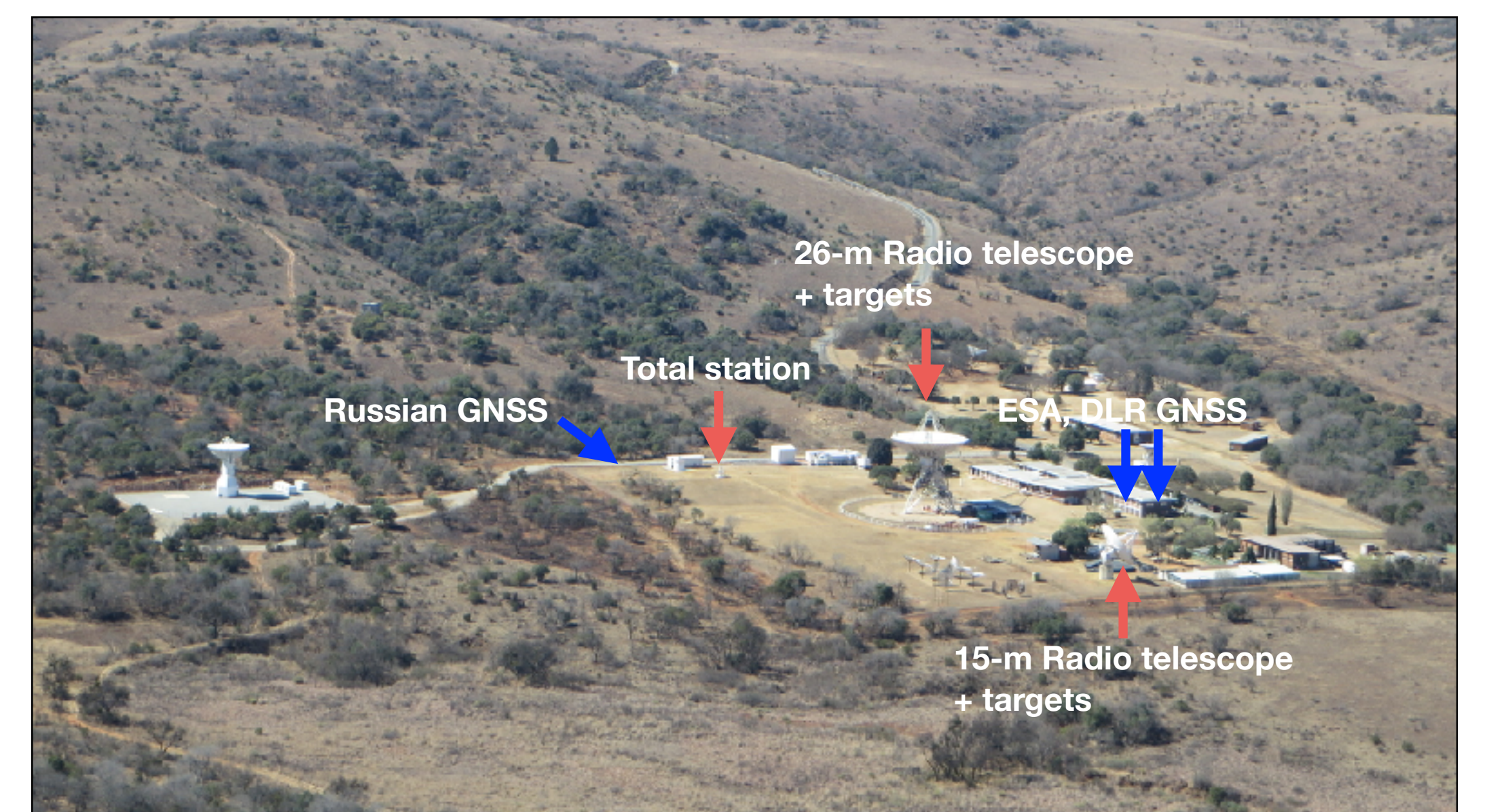
Figure 4: VLBI local tie observing system - components of measurement (red arrows) and reference (blue arrows) networks.
