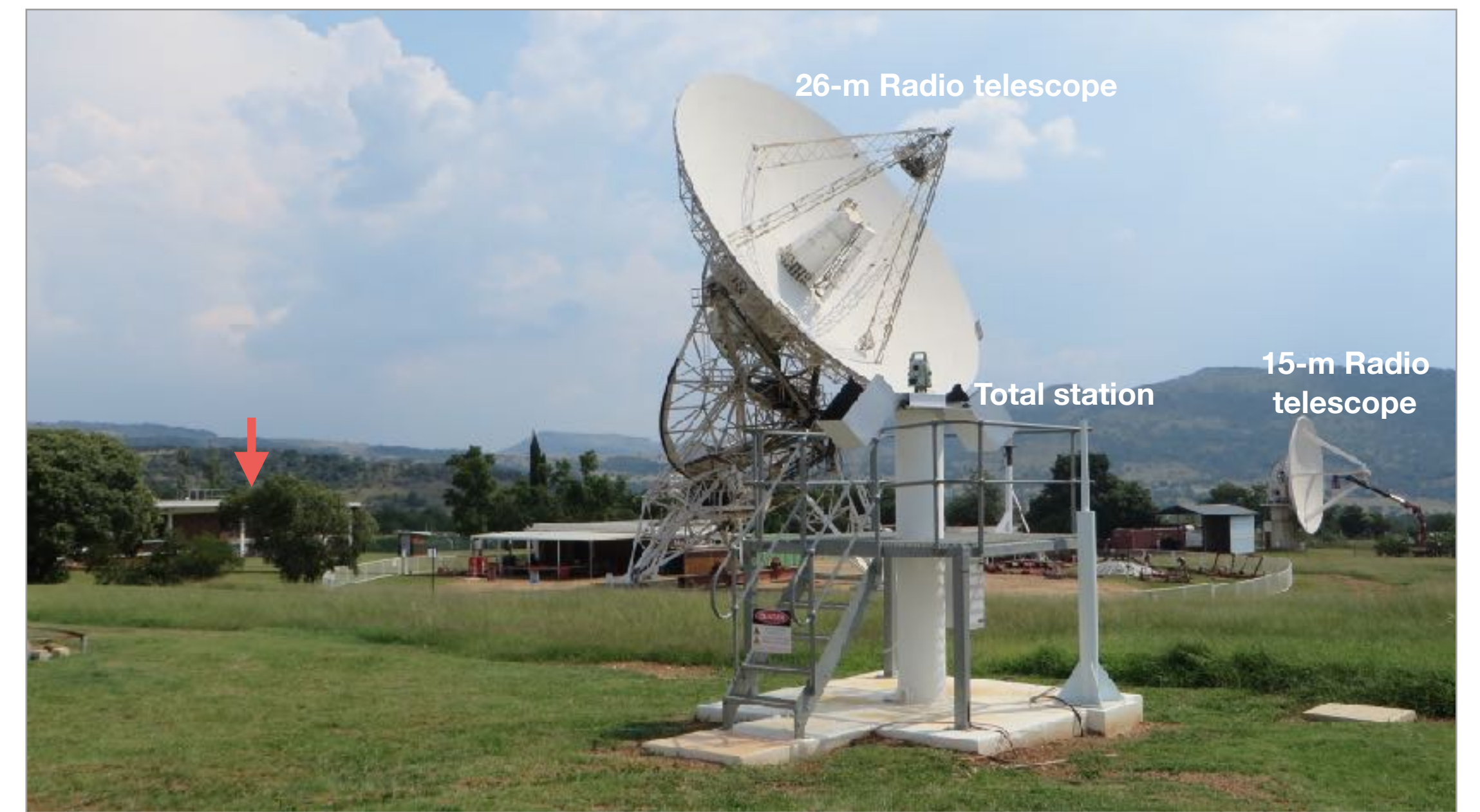
Figure 1: Short baseline of ~113 m between the HartRAO 26-m and 15-m antennas with the total station in the foreground. The planned position of a second total station installation on the roof of the control room for in-house ground survey / local tie measurements is indicated by the red arrow.
