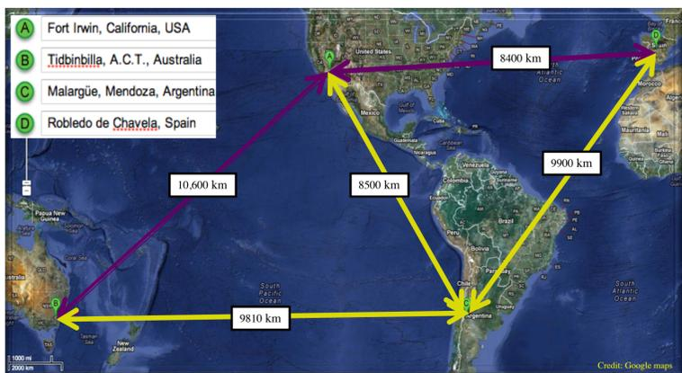
Fig. 1 NASA-ESA Ka-band network. The addition of ESA's Argentina station adds 3 baselines & Full Sky coverage. For  $\delta = +45$  to  $+90$  deg, only single California-Spain baseline. For  $\delta = -45$  to  $-90$  deg, only Australia-Argentina baseline.
