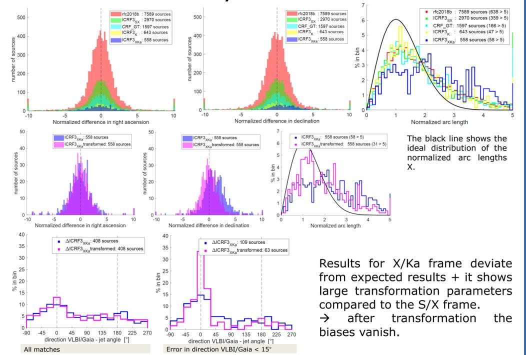
Results for X/Ka frame deviate from expected results + it shows large transformation parameters compared to the S/X frame.
