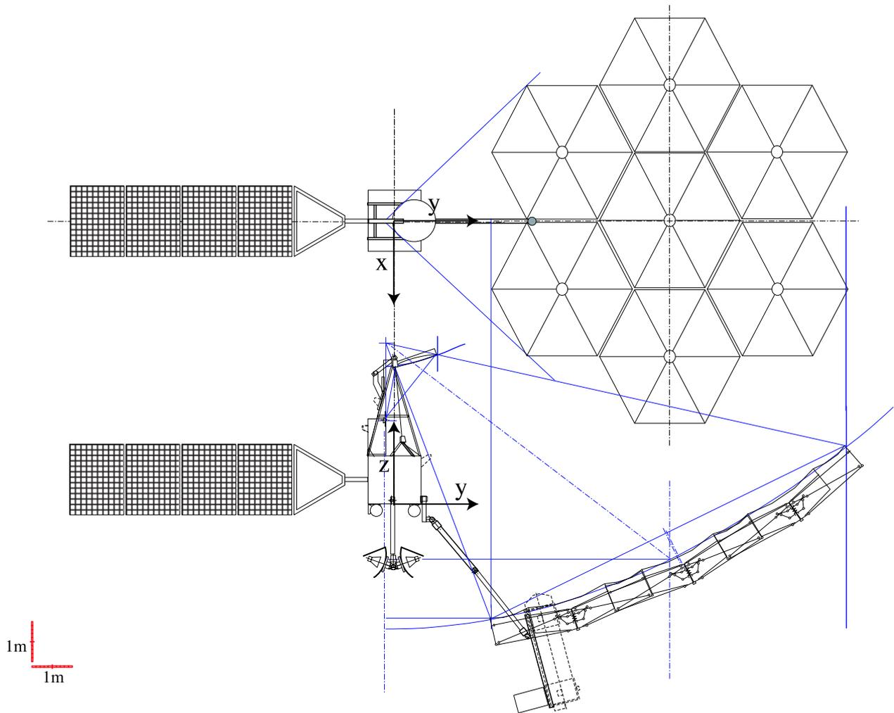
**Fig. 3.** The present design for the VSOP-2 spacecraft with a 9 m diameter offset Cassegrain antenna of seven hexagonal modules. The  $z$ -axis is along the antenna boresight direction. The main reflector, sub-reflector, high gain tracking station (“link”) antenna, and solar paddle are deployed in orbit. (Two link antennas are shown to illustrate the range of movement of this single antenna.)
