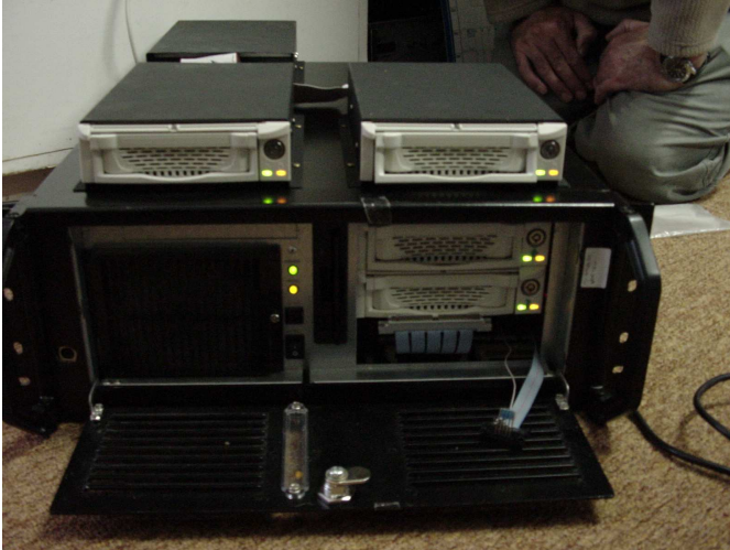
Fig. 1. The VLBI system for Ceduna with four demountable 200GB IDE drives. The VSIC connector is the 50 way ribbon connector at the bottom right.
