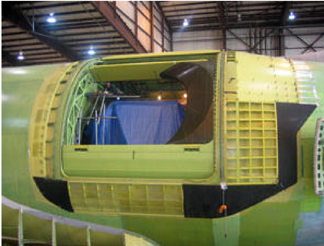
SOFIA Cavity Door Assembly installed on the B747 SP. Above the lower lip of the cavity, slats of the Lower Flexible Door (LFD) are seen where they attach to the Aperture Assembly (AA) which will track the telescope in elevation. At the aft (right side) of the cavity is the contoured ramp (dark brown), on which most of the air stream flowing over the cavity will reattach. The telescope is covered with a blue tarp. Some of the fuselage fairings around the cavity remain to be installed. This picture was taken in early May 2005.
