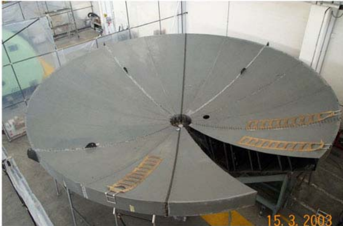
Figure 2. Status of the BUS as per 15.03.03. One slice (15) to be inserted
