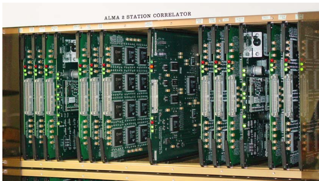
Figure 19. Fully populated prototype correlator station bin (no optical receiver cards).
