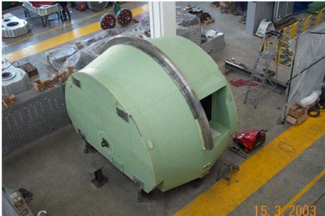
Figure 1. The cabin during painting (primer)
