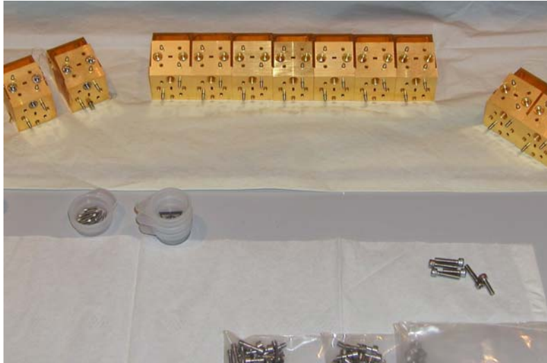
Figure 13. Band 3 orthomode transducers
