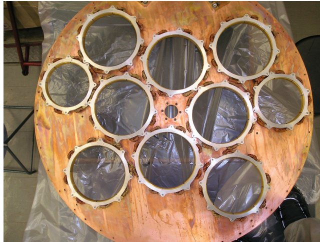
Figure 1 New 90 K plate with thermal links fitted
