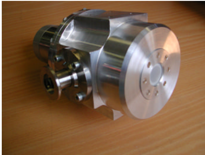
Figure 13. WVR cold load with Sterling cooler
