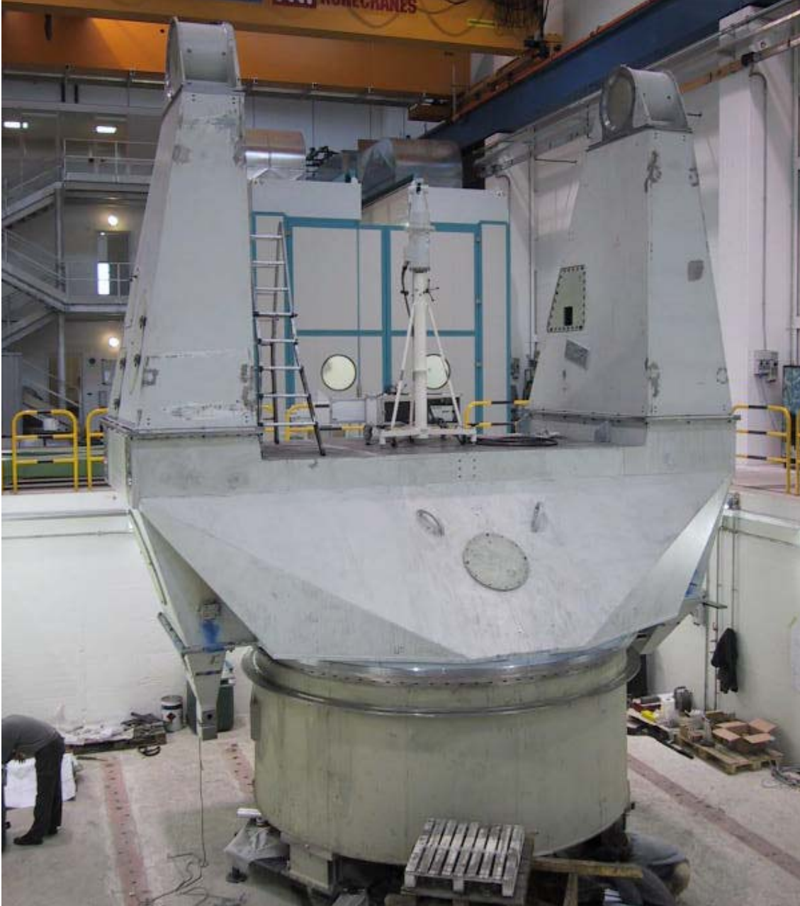
Figure 3. Mount structure during measurements of alignment with laser tracker.
