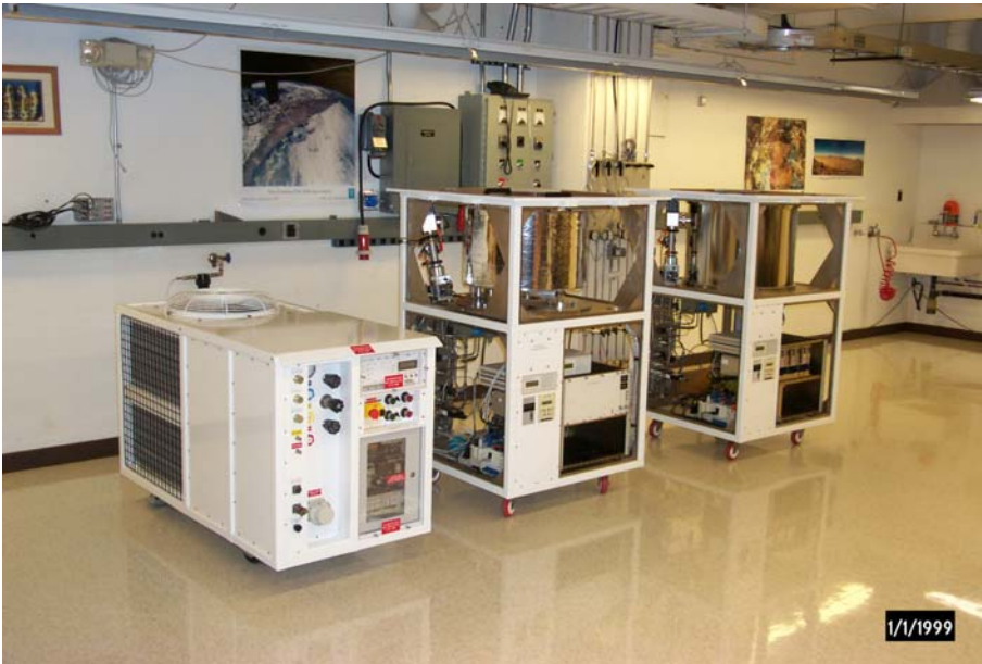
Figure 13. Cryostat compressor and two evaluation receivers.
