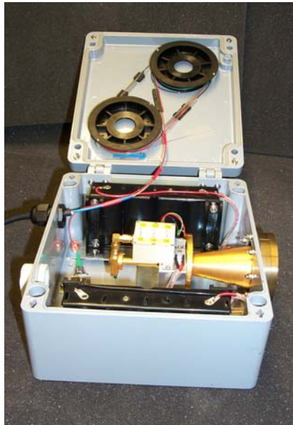
Figure11. Holography transmitter and receiver
