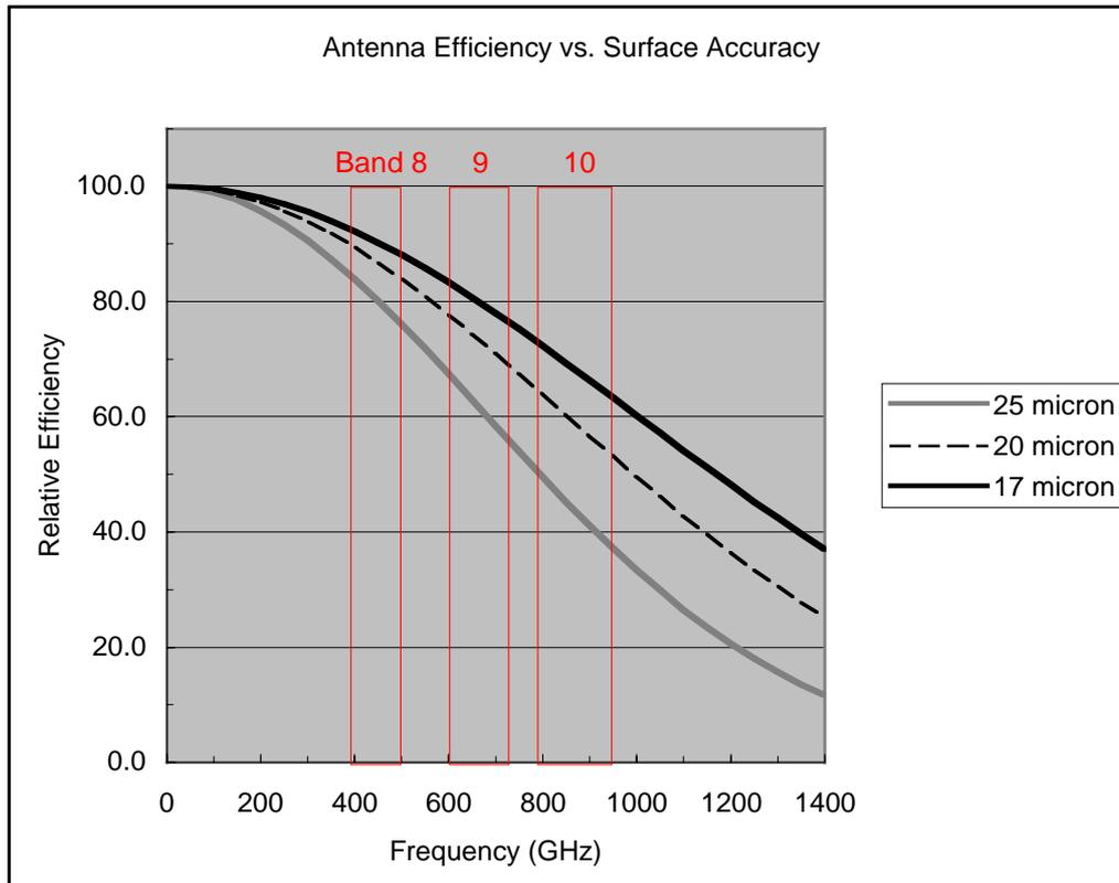
**Figure 4A: The relative efficiency of an antenna as a function of observing frequency.**
