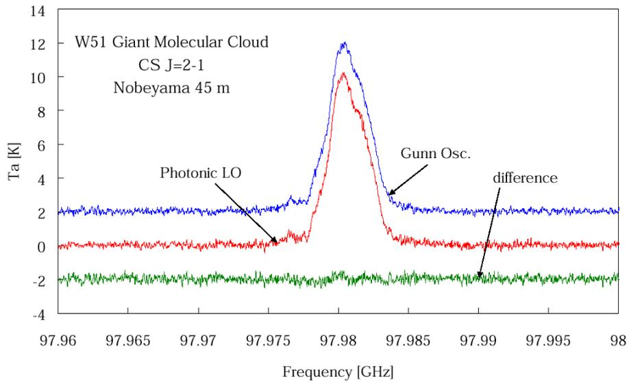
**Figure 5E:** (*upper*) The low noise high-power photomixer developed by NAOJ and NTT in Japan. (*lower*) Comparison of the spectral lines observed at the 45-m telescope at Nobeyama with a conventional Gunn oscillator as an LO (upper blue trace) and the photonic LO (middle red trace). The integration time is the same for both observations, and the results are virtually identical (lower green trace).
