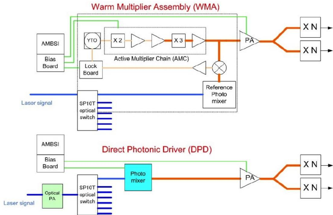
**Figure 5F: The block diagrams of the baseline (Warm Multiplier Assembly, upper) and the proposed hybrid-photonic (Direct Photonic Driver, lower) options for the ALMA local oscillator system. The hybrid option is much simpler than the current baseline system and is capable of evolving into a fully photonic LO system without multipliers with minimum cost.**
