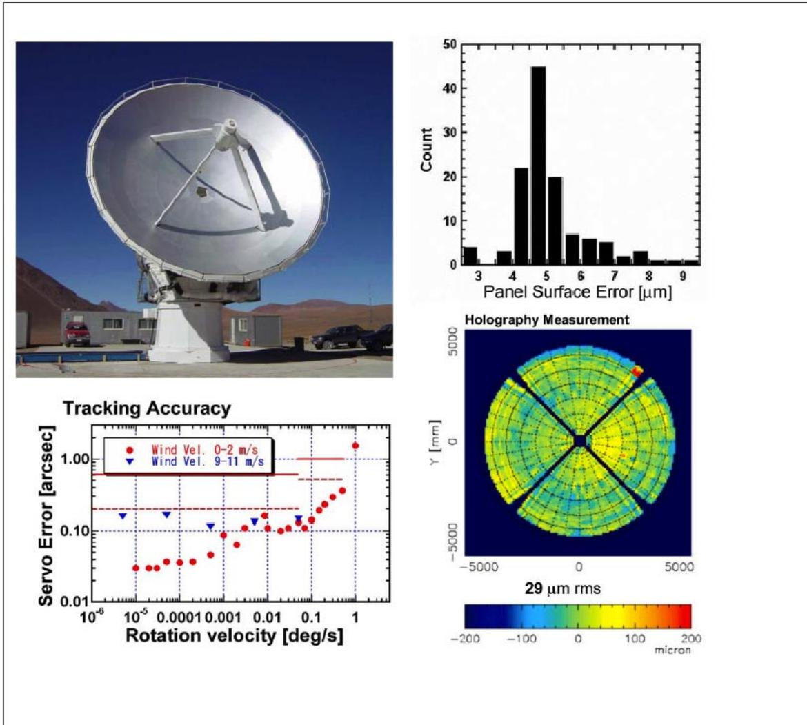
Figure 5A: The precision 10-m antenna installed at Pampa la Bola for ASTE, and its measured performances; tracking accuracy measured at Nobeyama (lower left), factory-measured panel surface errors (upper right), and the holographic measurement as of October, 2002.
