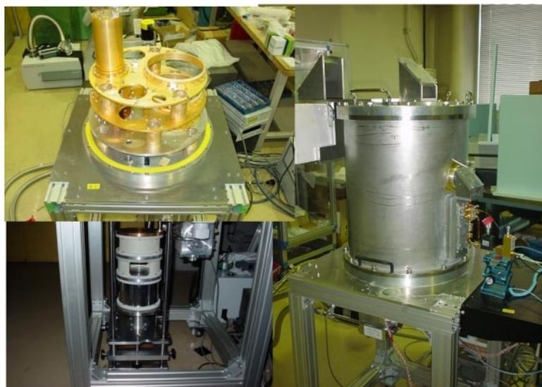
**Figure 5C: (*upper*) Receiver frontend cartridges under development for Band 4 (left), Band 8 (middle) and Band 10 (right). (*lower*) The cartridge test cryostat. Its copies are being shipped to the ALMA frontend development sites in Europe and North America.**
