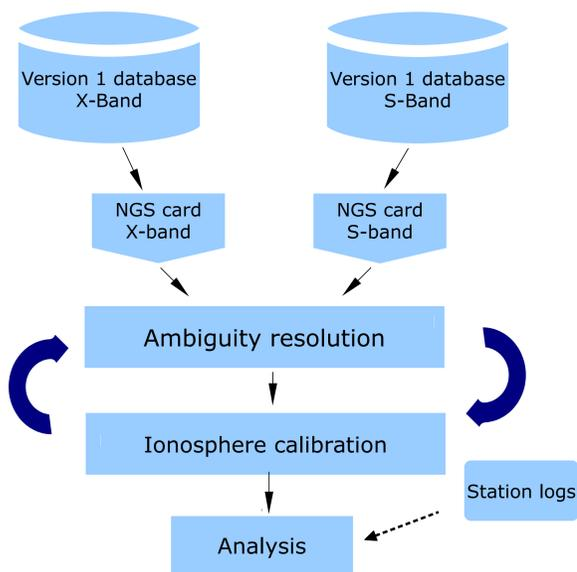
Figure 1: Flowchart of the automated data analysis with c5++.
